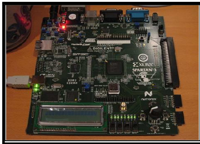
Fig. 10. Circuit Xilinx XC3S700A Spartan 3A Starter Kit
